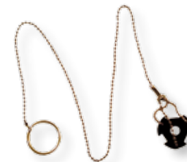
Photo 3. Simplified relascope with 3 chains and 3 apertures
