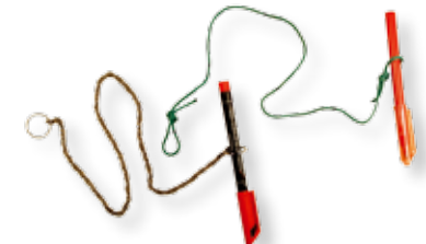
Photo 4. Self-made simplified relascopes
