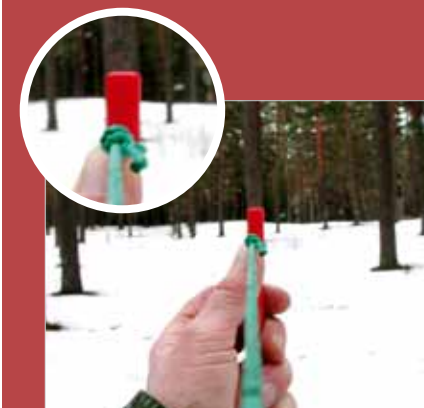
Photo 9. When it is difficult to decide whether the tree is seemingly thinner or thicker, 0.5 m^2/ha will be counted
